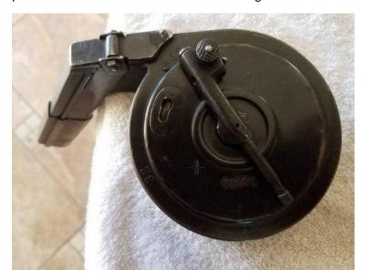
4a. Bing Brothers Telescoping Crank Bottom Plate With Retainer Through Bolt & Nut
