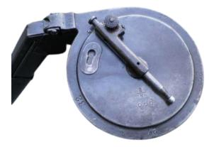
2a. Bing Brothers Telescoping Crank Bottom Plate With Retainer Screws
