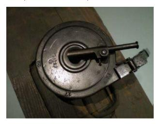
1a. AEG Telescoping Bottom Crank Plate With Reinforcing Ring
